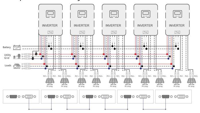
e. Six parallel-connected solar storage inverters:
