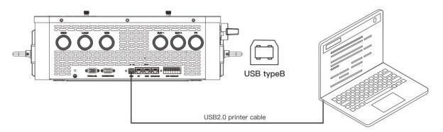
Users can use the upper computer software through the port to read and modify device parameters. If needing the installation package for the upper computer software, you can download it from the official website of SRNE, or contact us to get it.
